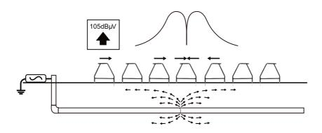
Eventually the A-frame will detect the fault signal and the "Fault Find" arrow will point forwards. Continue moving forwards, it may be worth reducing the distance between measurements points as the fault is neared.
