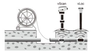
Adjust the sensitivity control so that the bar graph reads approximately 75%. Now move the locator forwards and back to detect the largest signal. You will also notice that there will be a "ghost signal" either side of the main signal. This is normal and characteristic of locating Sondes.
