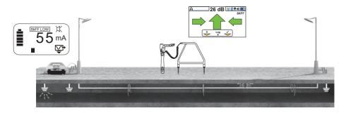
Plug in the analogue A-frame to the receiver accessory socket. When the receiver is switched on, it will automatically default to the A-frame screen.
