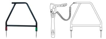
The vLoc3 series A-frame accessory is used to detect ground faults on pipes and cables. In the case of pipes, the faults consist of coating defects. In the case of cables, faults are usually caused by insulation damage allowing the metallic sheath (or internal conductor) to become in contact with the ground.
