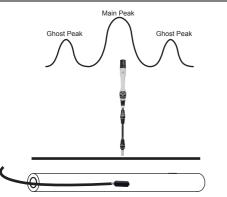
Now push the Sonde a couple of meters (yards) into the pipe. Stop and re-locate the Sonde. The direction of the Sonde can be confirmed by holding the locator vertically and rotating it on it's axis until the largest signal is detected. The Sonde will then be pointing at right angles to the display.
