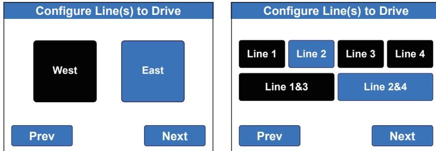
Figure 7-21 Configure Line(s) to Drive two ways (FLS-2-TX2W) and four ways (FLS-2-TX4W)
