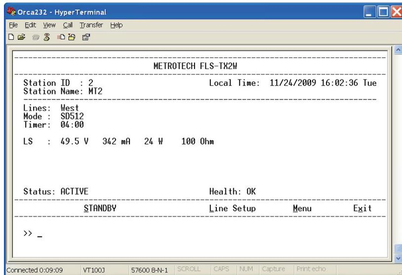
Figure 7-64 Main Operating Screen (Active Mode)
