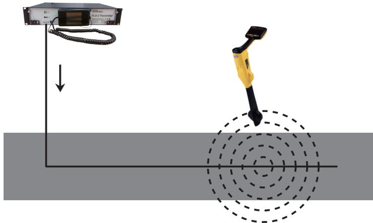
Figure 4-1 FLS-2 Transmitter and Receiver
