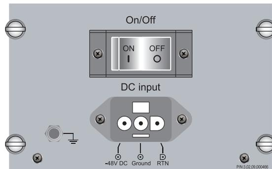
Figure 6-3 Rear DC Ground Connection of Ground Stud
