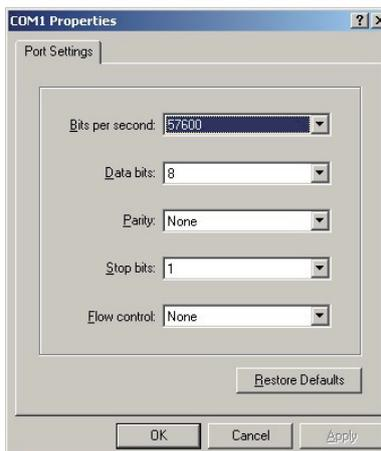
Figure 7-62 HyperTerminal Connection Properties
