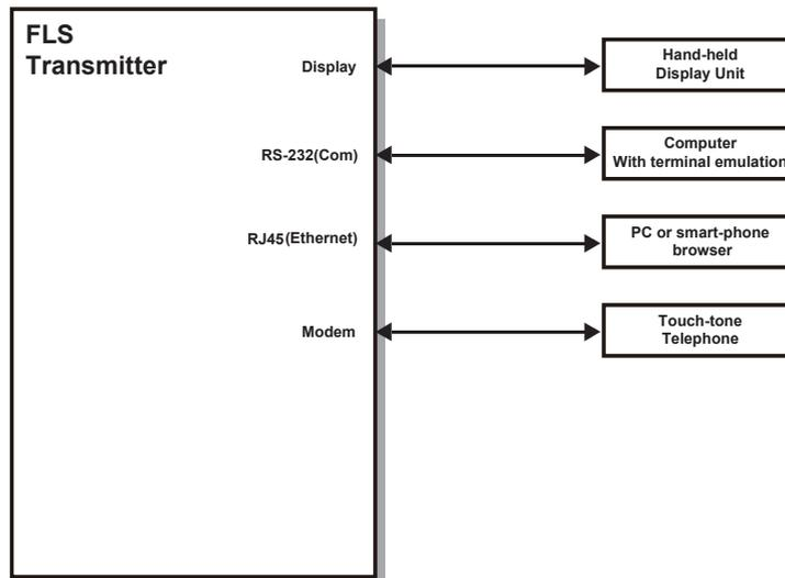
Figure 5-1 Methods of Controlling the Transmitter
