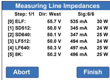
Figure 7-15 Measuring Line Impedances
