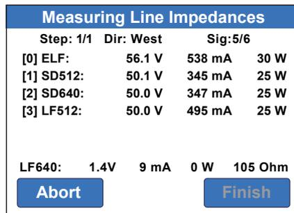
Figure 7-29 Measuring Line Impedances (Finish)
