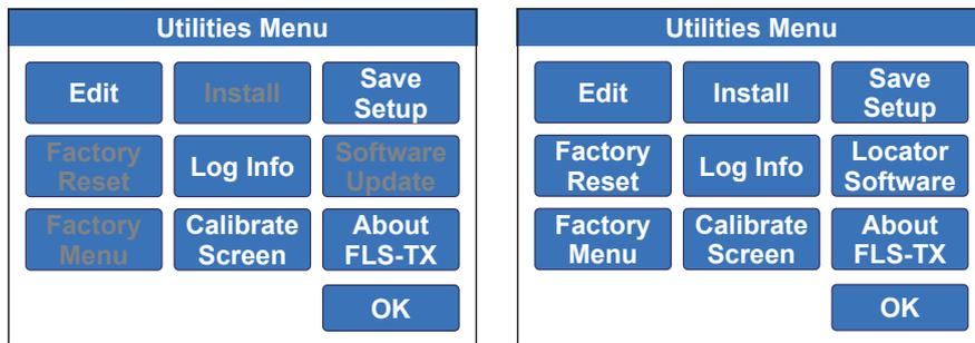
Figure 7-44 Utilities Menu (Active Mode and Standby Mode)
