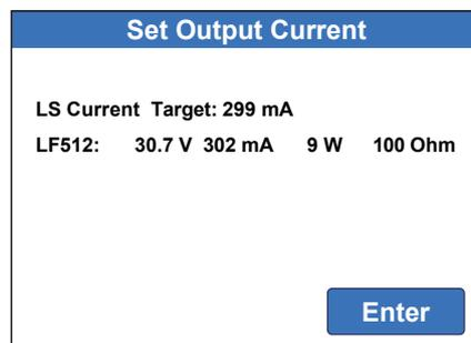
Figure 7-11 Set Output Current
