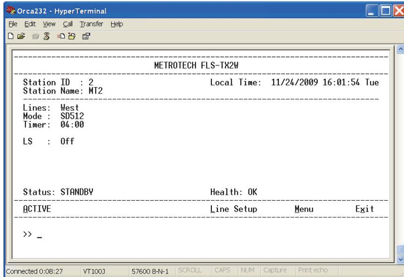
Figure 7-63 Main Operating Screen (Standby Mode)
