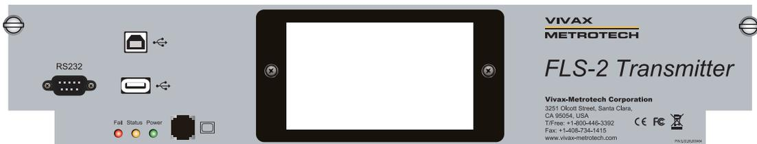
Figure 5-2 Main Control Module
