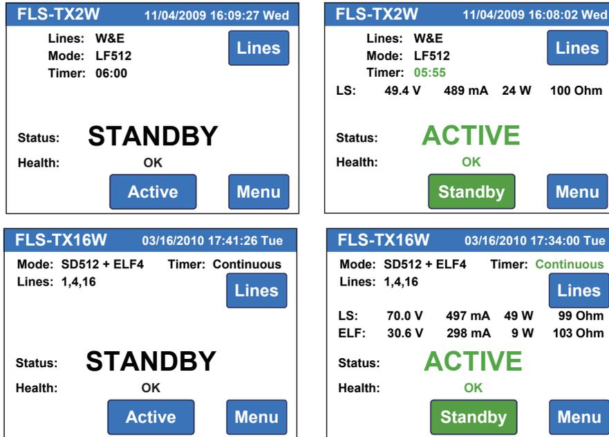
Figure 7-1 Main Operating Screen (Standby Mode and Active Mode)
