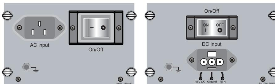
Figure 5-3 AC and DC Power Supply Module
