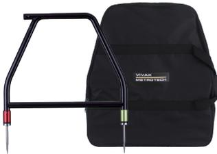
The A-frame accessory is used to detect ground faults on pipes and cables. In the case of pipes, the faults consist of coating defects. In the case of cables, faults are usually caused by insulation damage allowing the metallic sheath (or internal conductor) to become in contact with the ground.
