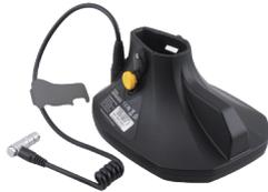
The plug-in adapter attaches to the bottom of vLoc3 series receivers for the purpose of locating buried EMS markers.
