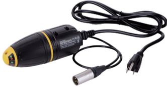
The LPC separation filter (LPC) is used to safely inject a trace tone to a live cable via a domestic mains socket, so that the cable can be traced from the premises to the connection in the street. It is suitable for connecting to voltages up to 250V AC.
