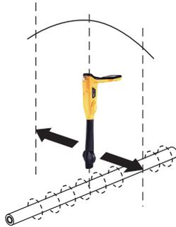
This uses a single horizontal antenna and provides a “Peak” or maximum signal response over the center of the buried line. The compass (line direction indicator) aligns itself parallel to the direction of the cable together with a line position indicator showing which side of the line the locator is (available in Active modes).
