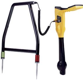
The analogue A-frame accessory is used to detect ground faults on pipes and cables. In the case of pipes, the faults consist of coating defects. In the case of cables, faults are usually caused by insulation damage allowing the metallic sheath (or internal conductor) to become in contact with the ground.
