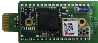
As an optional extra the vLoc3-5000 receiver can be fitted with a Bluetooth communications accessory. This allows communication with external GPS and or Dataloggers. The Bluetooth option can be retrofitted and can be ordered at a later date if preferred.
