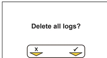
Press the "+" key to confirm. The locator will ask again "Are you sure?". Press the "-" key to delete or the "+" key to cancel the deletion and return to the locate/accessory screen.
