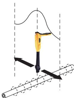
Two horizontal antennas provide a “Peak” or maximum signal response over the center of the buried line. The compass (line direction indicator) aligns itself parallel to the direction of the cable together with a line position indicator showing which side of the line the locator is (available in Active modes).
